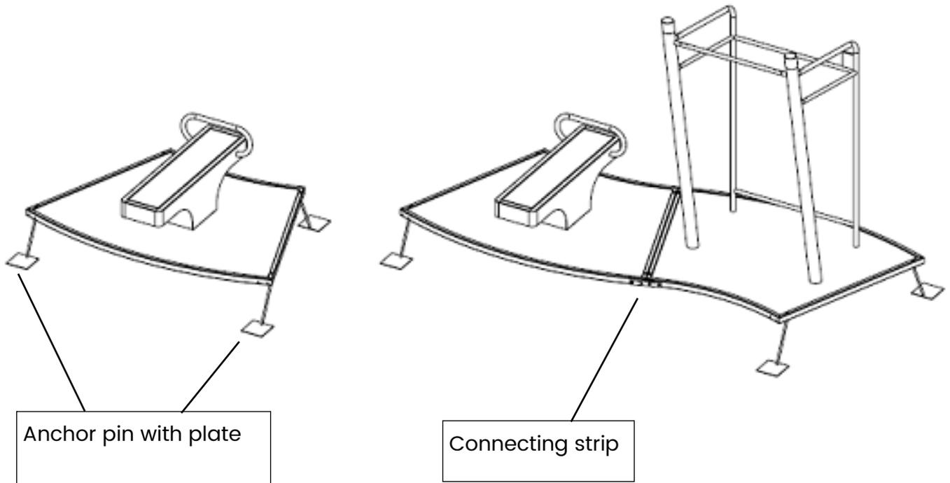
**When 3 or more floor parts are connected, anchoring in the ground (with anchor pin with plate) is NOT necessary.**
