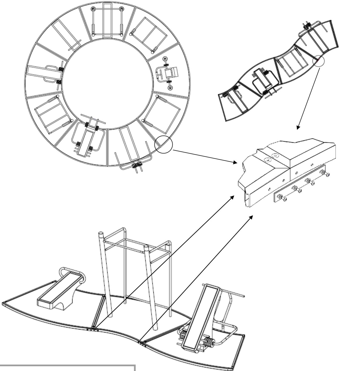
**When 3 or more floor parts are connected, anchoring in the ground is NOT necessary.**
